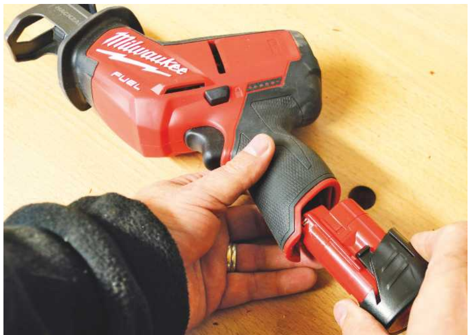
▲ Batteries slide into the handle. 4Ah ones are available for longer run times
